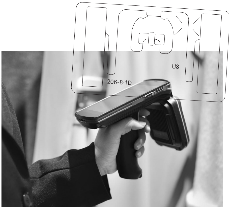
Handheld RFID-reader and RFID-tag UHF (Ultra-high frequency)
